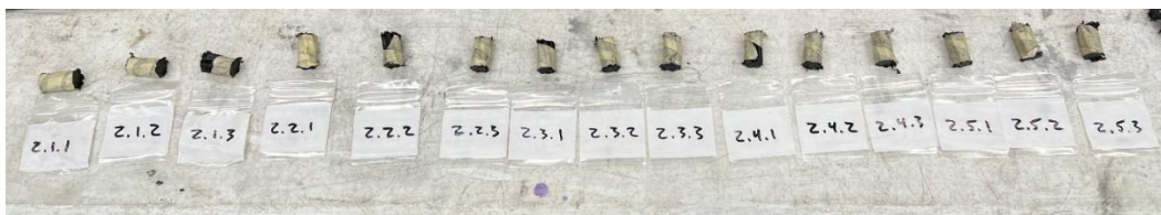
(b) Samples required for measuring water absorption per ASTM D570
