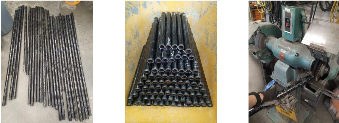
Figure A - 65. Steel pipes cut and deburred
