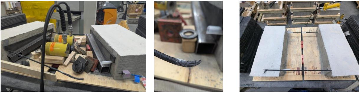
Figure A - 53. Successful failure at the bend location – Phase 2
