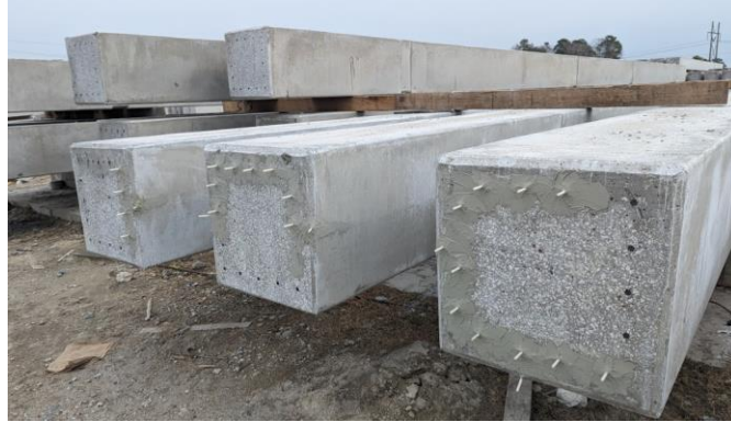
Figure A - 11. 24 in. CFRP-prestressed square piles
