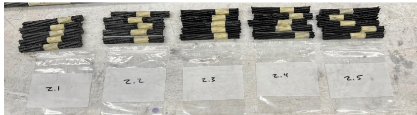
(a) Samples required for measuring the cross-sectional area per ASTM D792
