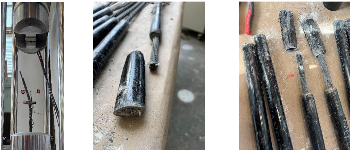
Figure A - 68. Pipe rupture as a premature failure mode
