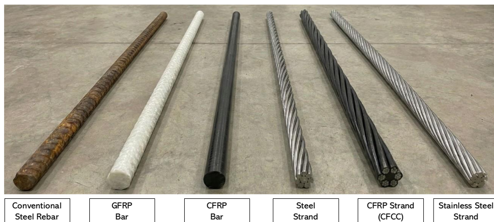
Figure 2. Reinforcement bar types
