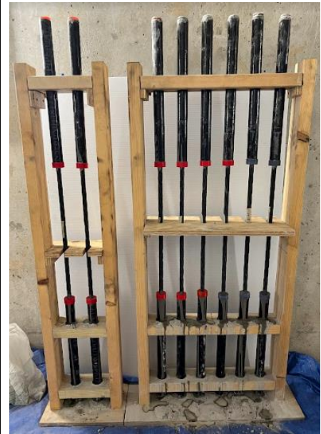
(e) Alignment fixture
