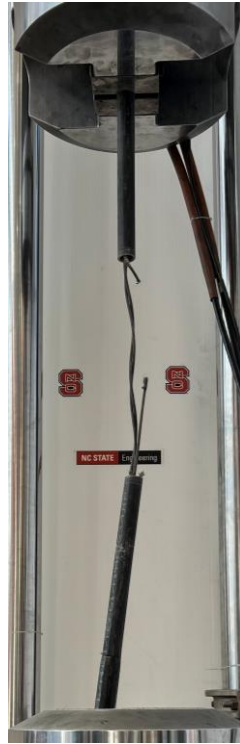
Figure A - 70. King wire remaining after CFRP strand failure
