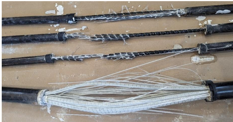
Figure 16. GFRP bars after failure
